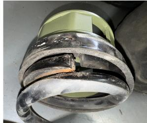
Step 10. Using a floor jack, compress spring by lifting on the lower arm until the lower control arm can be reinstalled. Use a screwdriver to position the hub so that the bolt holes line up. (see photo) Leave these bolts loose until vehicle is on the ground in a later step.
