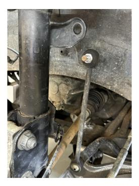
Step 7. Remove bolts connecting strut to hub and remove strut (see photo) Save hardware for reinstallation. If installing camber adjustment bolts, only one original bolt from each side will be reused.
