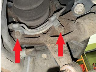
Step 4. Support rear lower control arm with floor jack. (Under the spring)
