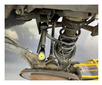
Step 12. Reinstall ABS wiring and reconnect sway bar link. Torque sway bar link nuts to 44 ft-lb.
