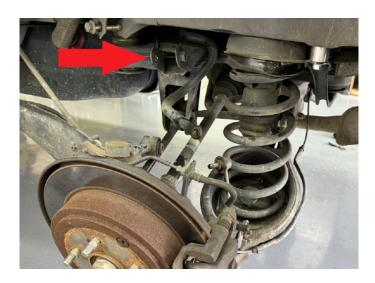
Step 2. Remove cotter pin and nut holding upper control arm to hub. Strike with heavy hammer to release arm from hub. Remove and discard OEM rear upper control arm.
