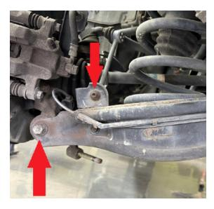
Step 7. Use the floor jack to release pressure on the spring.
