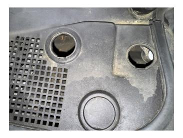
Step 2. Remove nuts holding struts to body, leave one nut on so struts do not fall when lifting vehicle to access bottom bolts. Save hardware.
