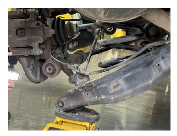
Step 8. Remove spring and rubber isolator.
