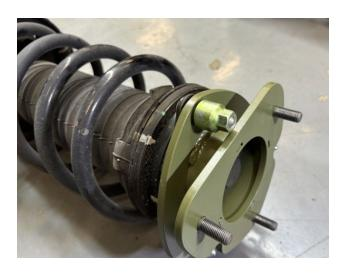
Step 10. Reinstall strut, using supplied hardware to bolt strut to body. Tighten mounting nuts to 33 ft-lb. This process is made easier by pulling up the plastic cowl cover.
