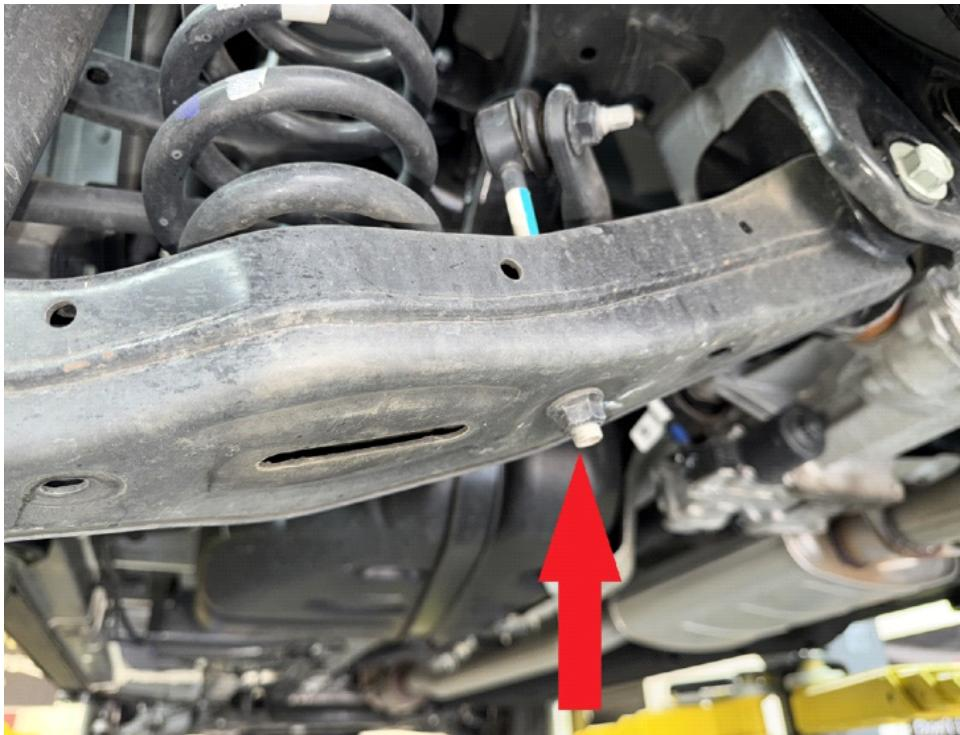
Step 6. Support lower control arm with hydraulic floor jack.
