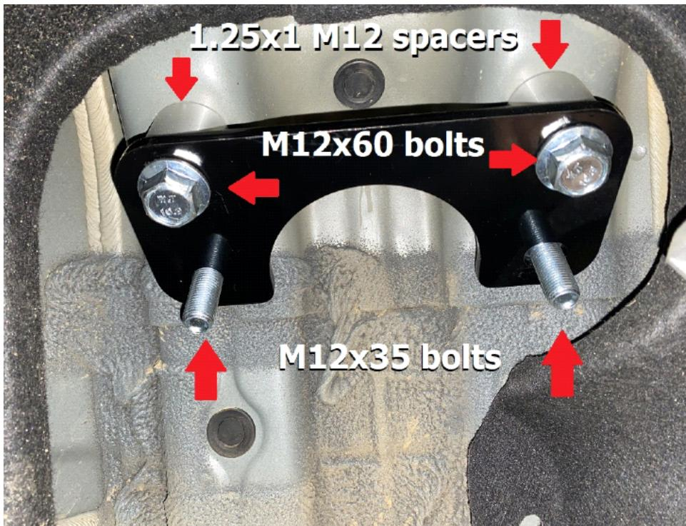
Step 13. Install rear shock absorber as shown:
