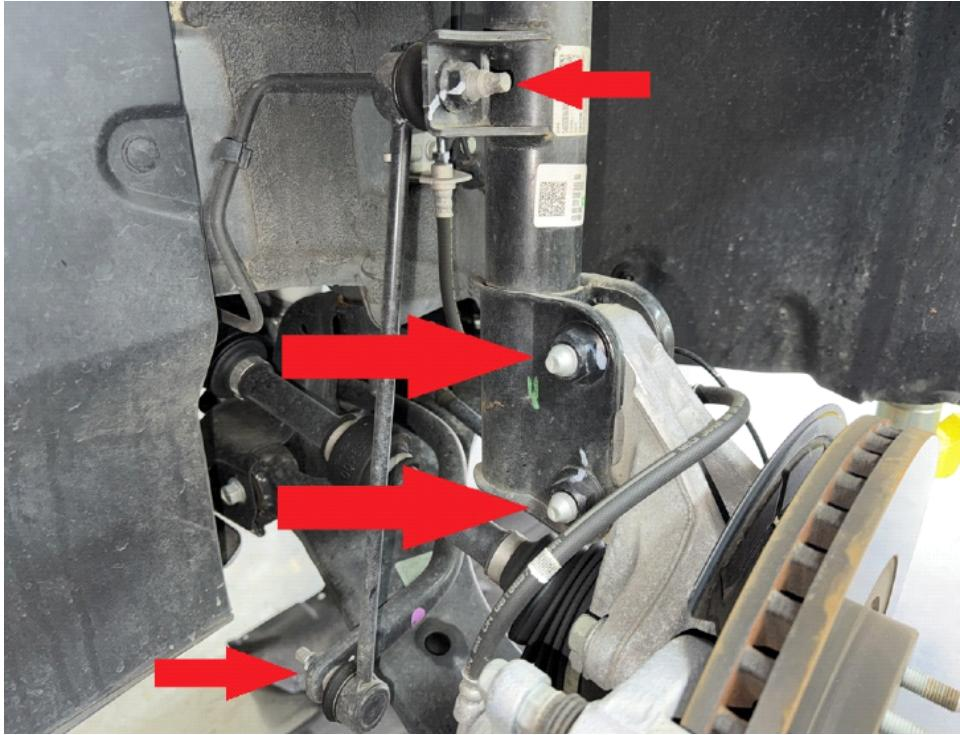
***NOTE: Do not allow the hub to fall loose, as the axle may come out of the inner CV joint.***
