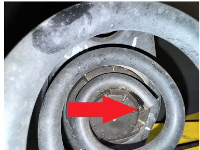
Step 19. Using a jack, lift lower control arm until shock bolt holes line up.
