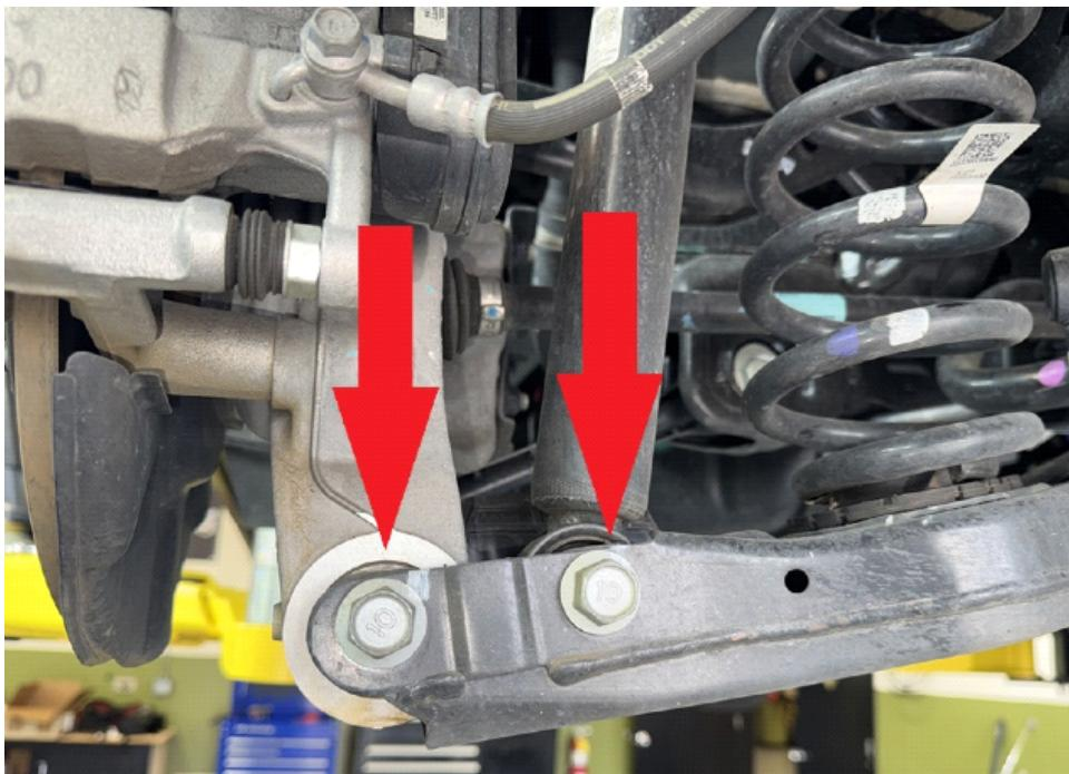
Step 9. Carefully release spring pressure by lowering floor jack.
