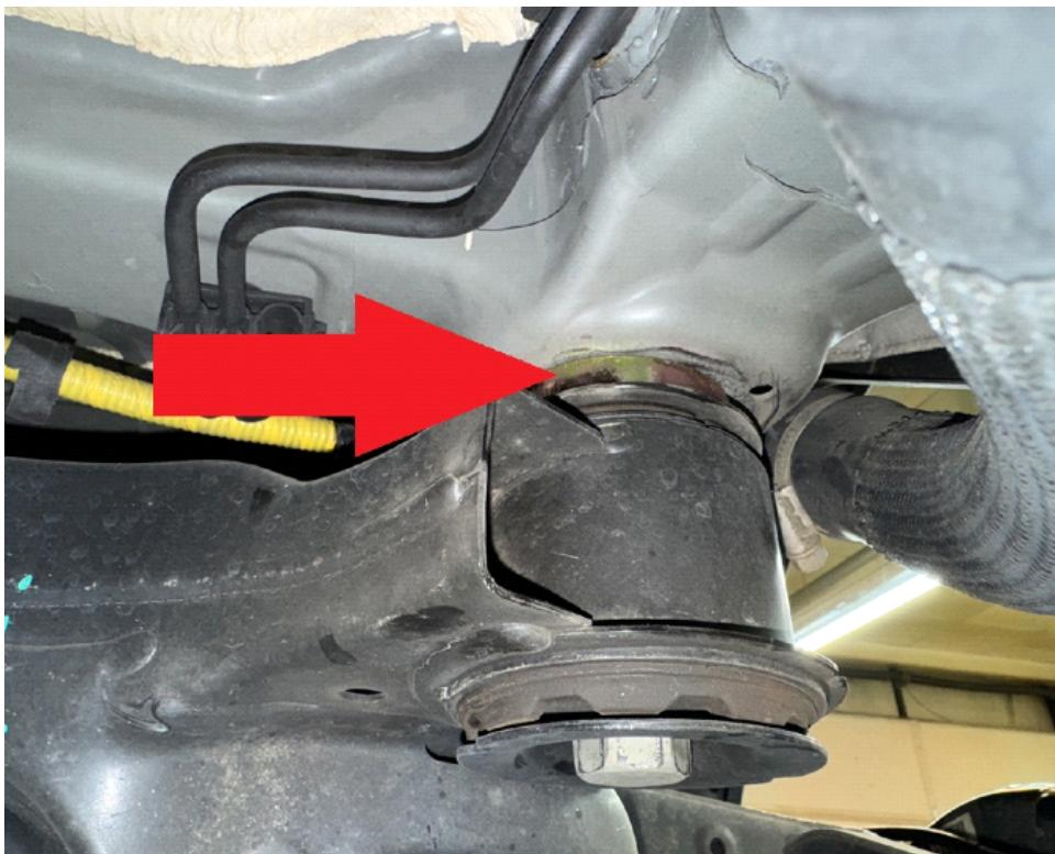
Step 28. Place 2 "C" spacers between subframe and body on REAR 2 studs. Tighten nuts.
