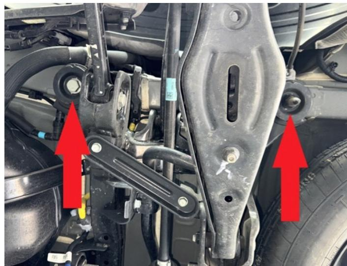
Step 27. Place 2 "G" spacers between subframe and body on FRONT 2 bolts. Tighten bolts.
