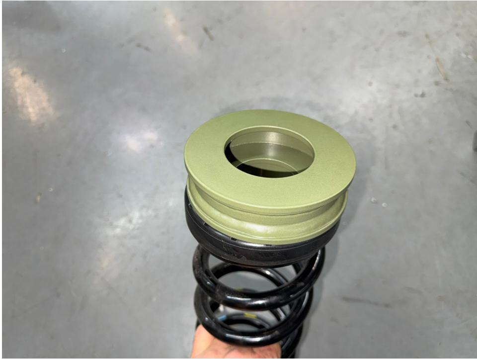
Step 18. Install spring and spacer. Be sure to rotate the spring so that it fits neatly in the relief cut in the lower rubber isolator. (see photos)
