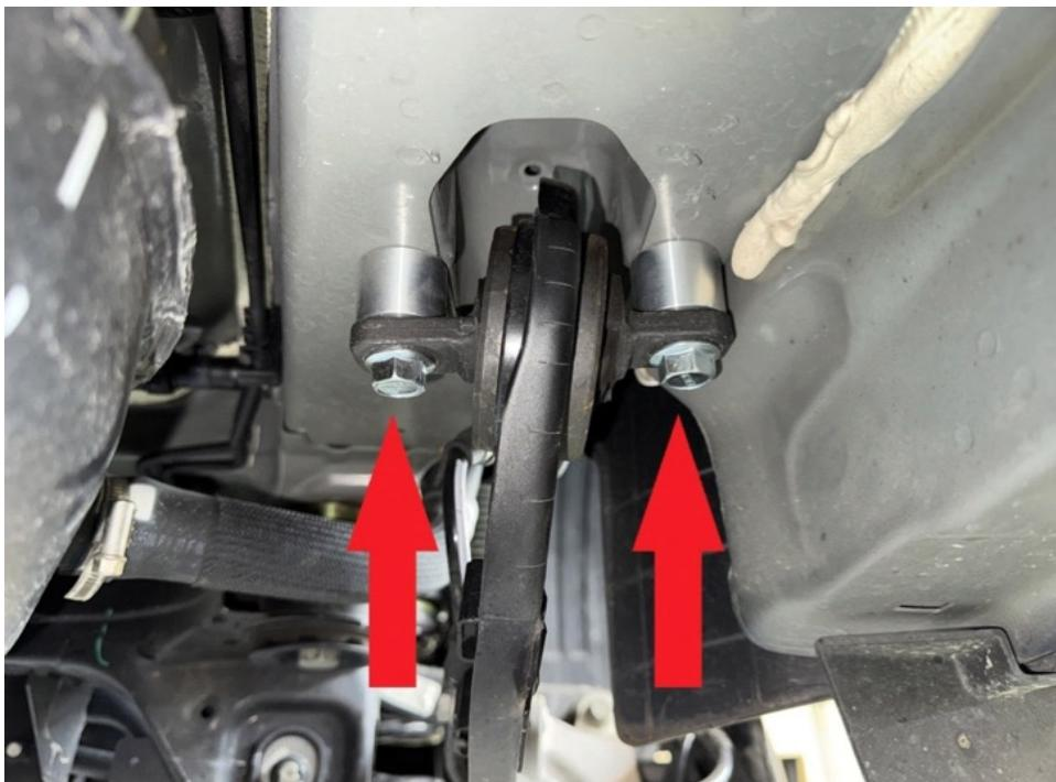
Step 17. Place rubber isolator over rear spring spacer.
