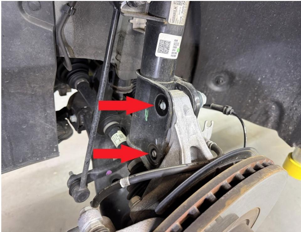
Step 11. Reinstall bolt holding brake and ABS lines.
