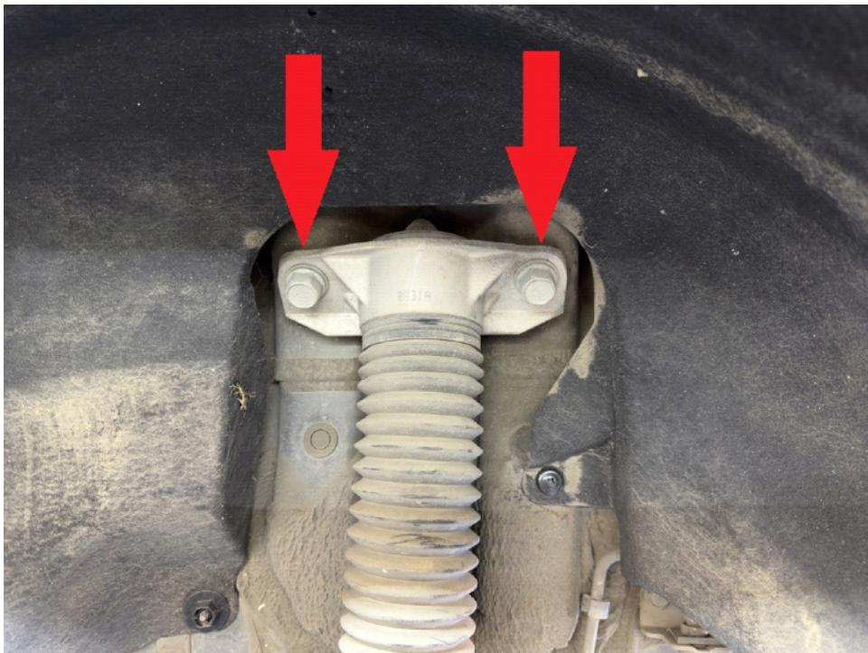
Step 12. Install rear shock relocation bracket as shown:
