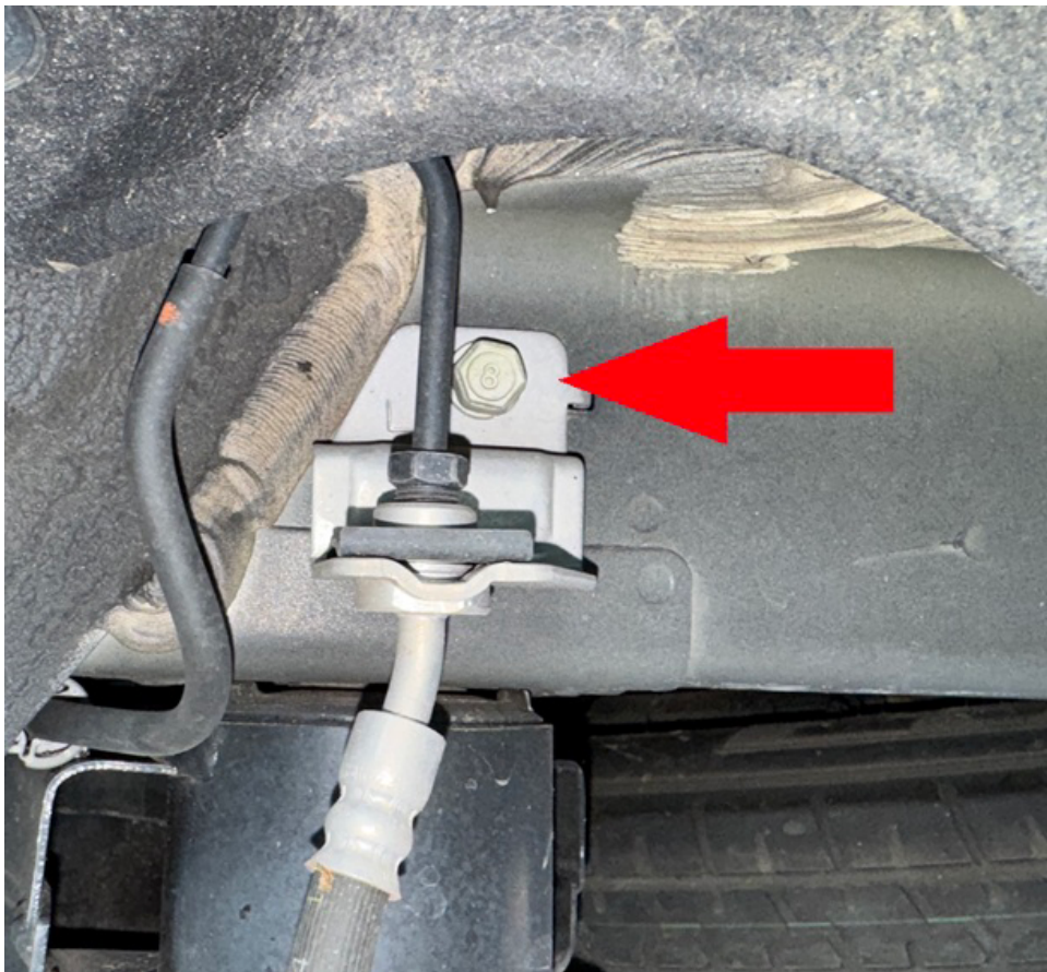
Step 5. Install brake line relocation bracket as shown:
