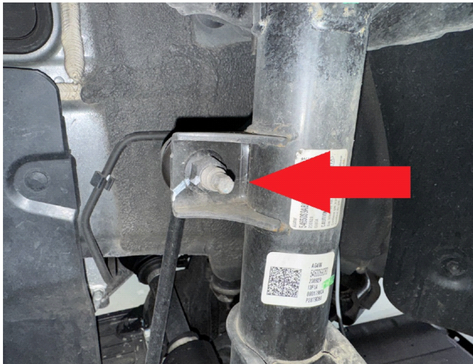
Step 5. Remove nuts connecting strut to knuckle. Tap bolts out with a hammer.
