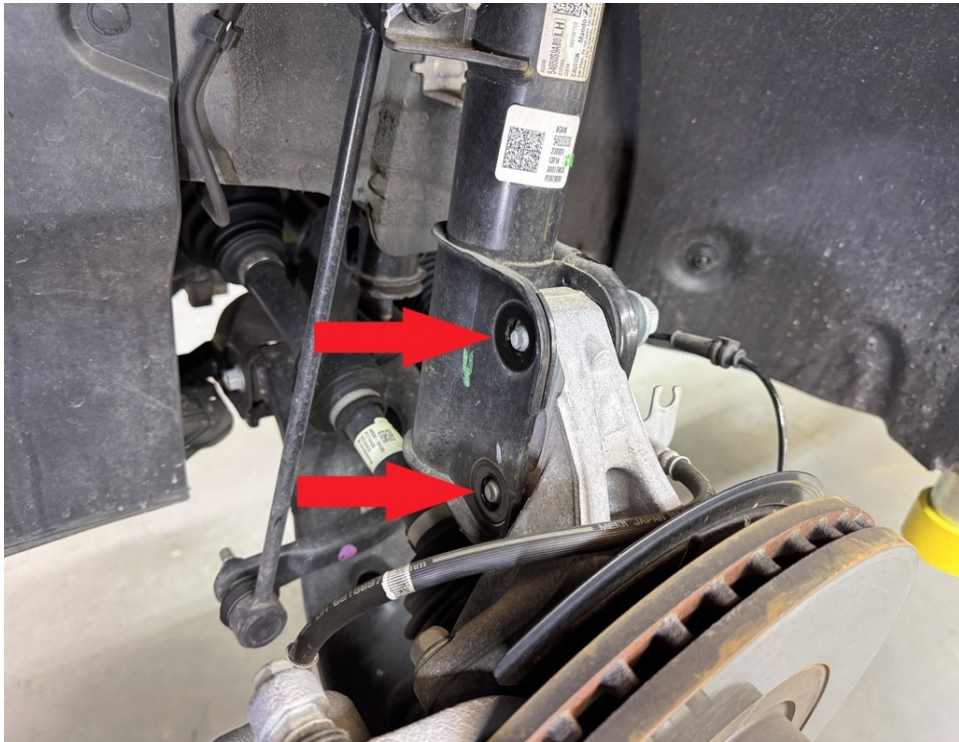
Step 11. Install offset camber adjustment bolt in place of upper strut bolt. (see separate instructions on last page.)
