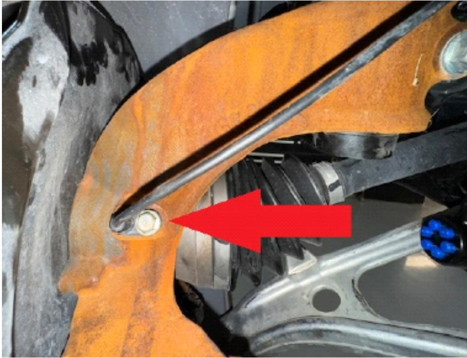
Step 5. Remove nut holding tie rod end to hub, strike knuckle with heavy hammer to dislodge tie rod end.
