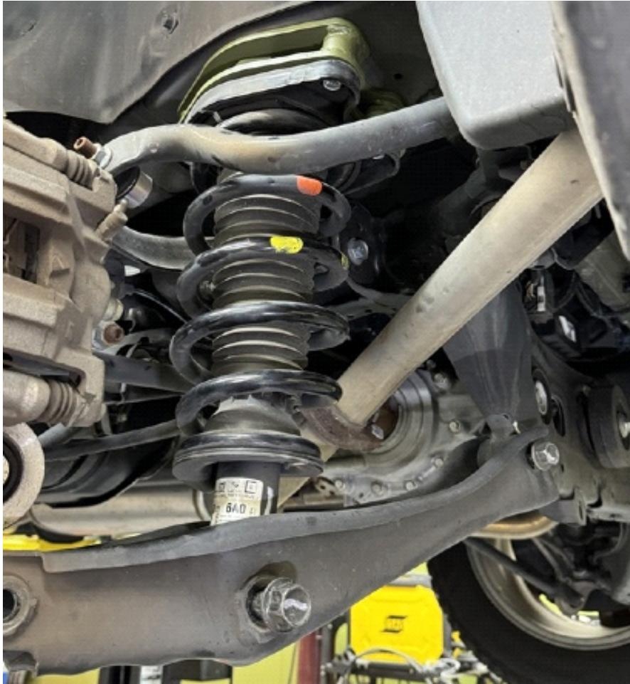
Step 10. Using a floor jack, lift up on lower control arm until bolt holes line up.
