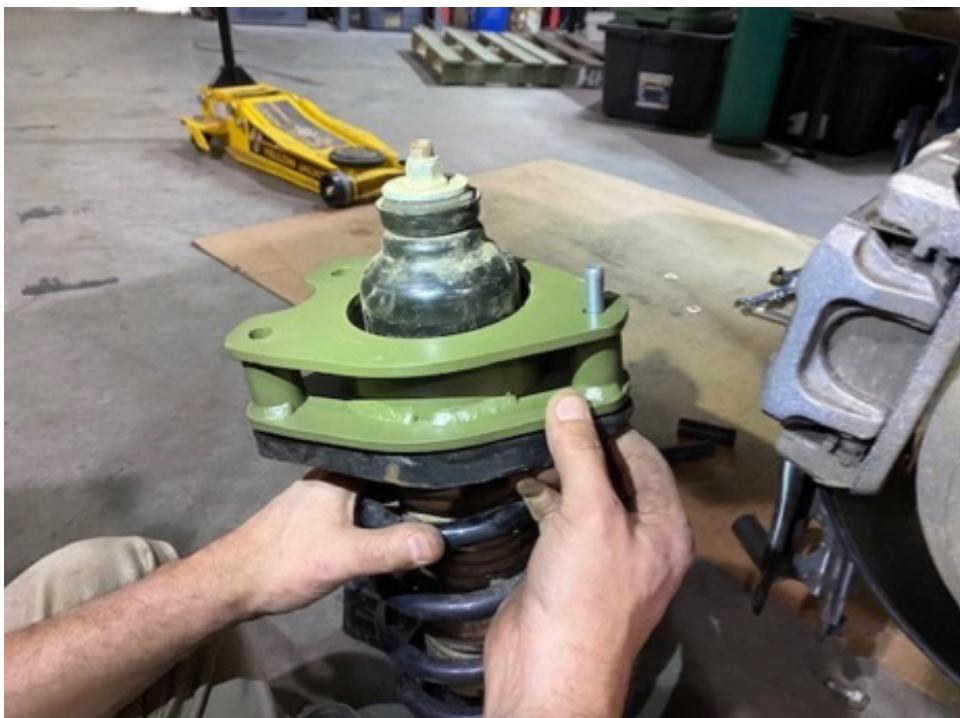
Step 8. Install strut/spacer combination using supplied hardware. Torque bolts to 44 ft-lb. BE CAREFUL NOT TO CROSS THREAD THESE BOLTS!
