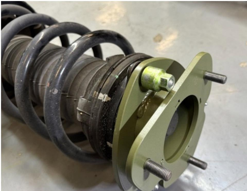
Step 15. Reinstall strut in reverse order, using supplied hardware (M10 nuts) to secure strut to body.
