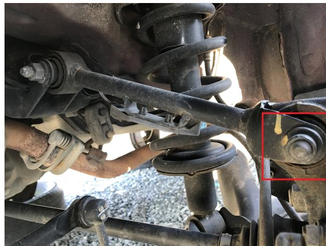
Step 4. Remove 19mm bolt connecting rear strut to lower arm.
