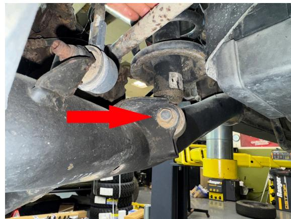
***Note: These bolts are prone to seizing inside the bushing. If the bolts seize, you will need to cut the bushings out and replace them or replace the strut.***
