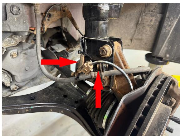
Step 4. Remove the castle nut and strike the steering arm with a heavy hammer to dislodge the tie rod end. Save hardware.
