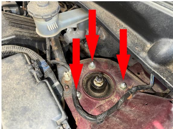
Step 7. Install lift spacers onto struts using original hardware as shown:
