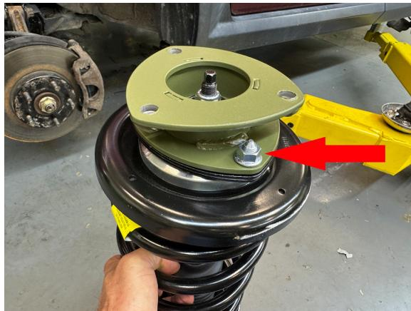
Step 8. Rotate the top of the strut 180° to line up spacer.
