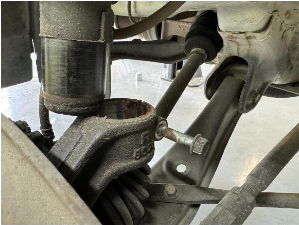
Step 13. Remove driver side strut.
