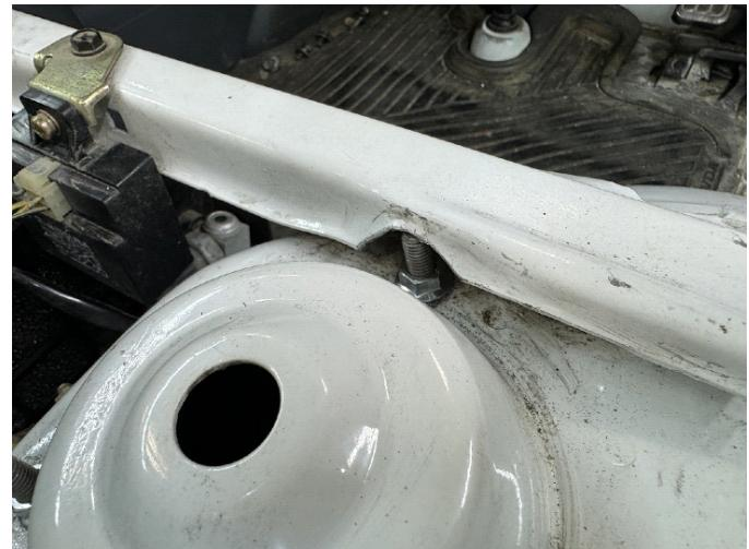
Step 16. Slide strut back into place with the "R" (DRIVER SIDE) as shown in photo and install the original 12mm nuts. The flat edge of the spacer goes toward the back of the vehicle. torque strut mounting nuts to 25 ft-lb.
