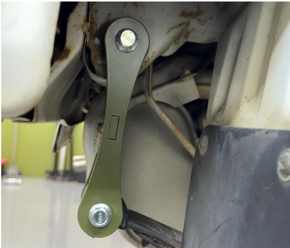
Step 9. Remove 2 12mm bolts holding driver side (RIGHT) shock absorber to body. Step 10. Place 2 1.5" long x 0.75" diameter aluminum spacers between shock absorber and body, secure in place with 2 M8x60 bolts. Torque to 25 ft-lb.
