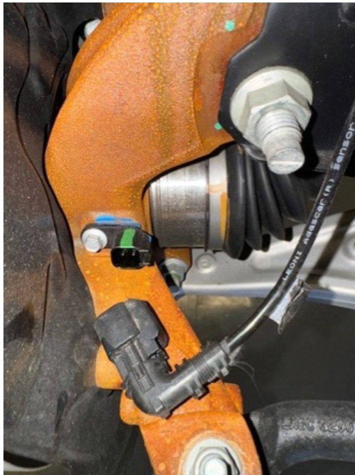
Step 13. Remove subframe mounting bolt with the star shaped washer.
