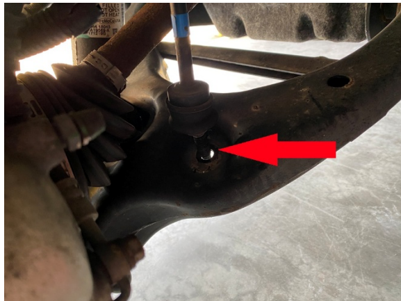
Step 7. Remove nut holding sway bar end link. Newer models shown on left, older models shown on right.
