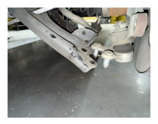
Step 14. Drill sway bar mounting holes for sway bar link 1/2"
