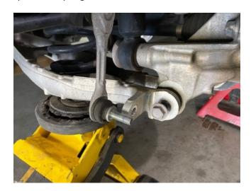
Step 21. Reinstall bolt holding lower control arm to wheel hub.
