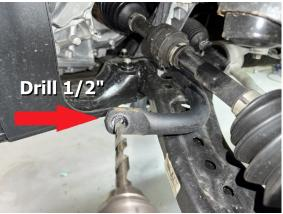
Step 15. Install new sway bar link. Note: sway bar link holes will not line up until both sides are lifted.
