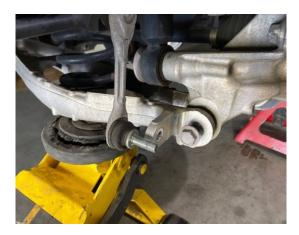
Step 17. Remove spring and place lift spacer on top of rubber isolator as shown.
