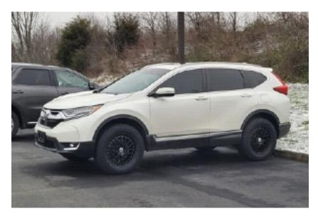
Note: Installing a lift kit will change the suspension geometry and will require a 4-wheel alignment.
