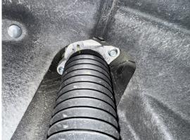
Step 20. Use jack to compress the spring and raise the lower control arm back into place.
