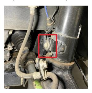
Step 5. Remove nut and cotter pin, strike knuckle to release tie rod end.
