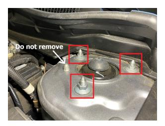
Step 10. Place strut spacer on top of strut and secure with hardware provided in the kit.
