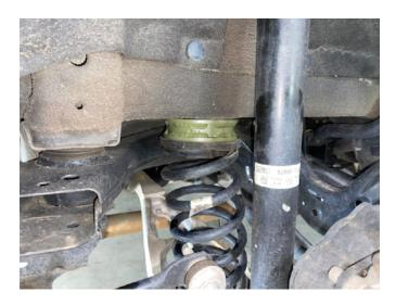
Step 19. Place rear shock spacer between rear shock and body, install M8x60 bolts. torque bolts to 30 ft-lb
