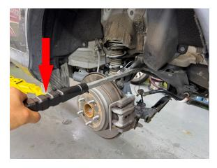
Step 20. Install adjustable upper control arm at this time (optional). Adjust arms to be slightly longer than the OEM arms. (Alignment technician will make final adjustments)
