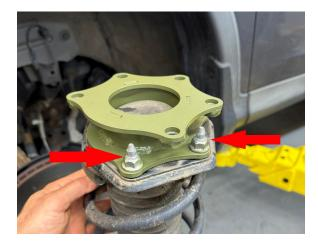
Step 10. Reinstall strut to shock tower using supplied M10x25mm bolts. Torque nuts to 33 ft-lb.
