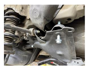
Step 12. Remove M12x100 bolt from previous steps and place 1.25x1 M12 spacer between subframe and chassis on driver side front corner. Permanently install bolt. Repeat for the remaining 3 subframe bolts. Torque to 76 ft-lb.
