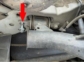
Step 7. Place 1.25x1 M12 spacers between trailing arm and chassis. Permanently install M12x80 bolts. Repeat trailing arm procedure on passenger side. Torque bolts to 76 ft-lb.
