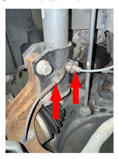
Step 4. Remove bolts connecting strut to knuckle. Save hardware for reinstallation.
