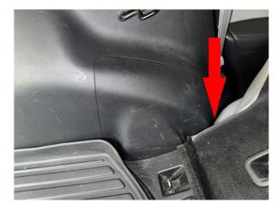
Step 2. Locate and remove strut mounting nuts. (save hardware)
