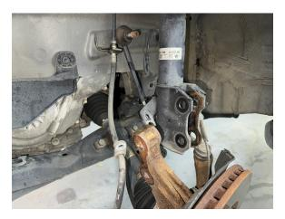
Step 7. Remove plastic panels to gain access to strut mounting bolts..
