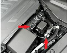
Step 11. Remove bolts holding driver side strut to shock tower (CX-90 shown).
