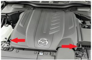
Step 9. Remove 2 10mm bolts holding the air duct to the radiator support.
