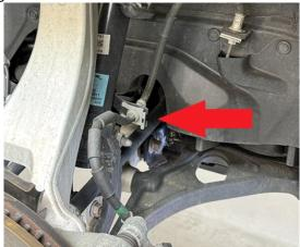
Step 4. Remove bolts holding strut fork to strut and lower control arm.
