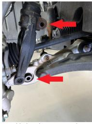
Step 5. Remove bolt holding sway bar end link to lower control arm.
