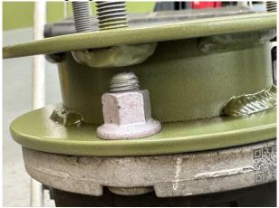
Step 14. Position strut back in shock tower, and loosely install 3 M10 nuts included in the kit to hold it in place but allow some movement until the installation is complete.
