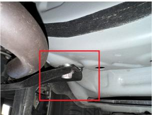
Step 25. Locate 19mm nuts on main subframe studs, loosen, do not remove both rear nuts, allowing subframe to drop about ¼ inch (6.3mm)
