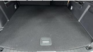
Step 2. Remove rearmost cargo tray and storage compartments.
