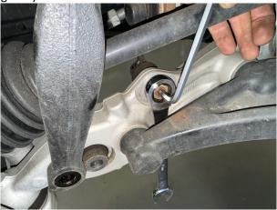
Step 6. Push suspension assembly downward to release strut fork from lower control arm.
