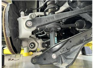
Step 12. Remove lower rear strut bolt.
