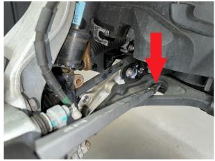
Step 16. Tap the strut fork with a heavy hammer so it can slide all the way back on. Be sure tab on back of strut lines up with gap in back of strut fork!
