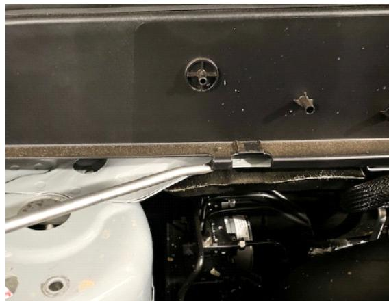
Step 7a (HYBRID MODELS ONLY) unclip wiring harness from cowl cover.
