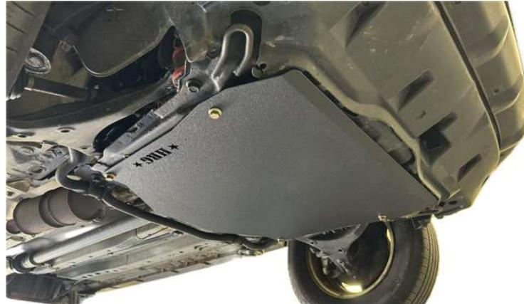
Step 5. Tighten bolts with 5/8" socket. Do not overtighten bolts!
