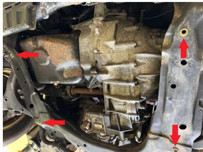
Step 4. Place skid plate under vehicle and secure with 4 1" long x 1/2" bolts.
