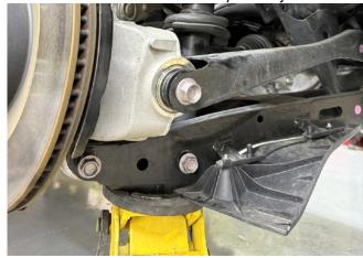
Step 10. Loosen bolt holding lower control arm to wheel hub.
