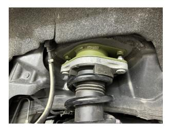
Step 18. Install nuts holding strut/spacer combo under rear seat using hardware provided in the kit. Step 19. Using a hydraulic jack, compress rear strut while **pushing the lower control arm forward** to line up the bolt holes on the wheel hub.
