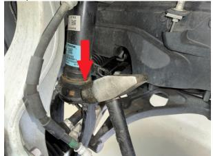
Step 9. Once strut and strut fork are separated, remove 3 nuts on the shock tower holding the strut in.
