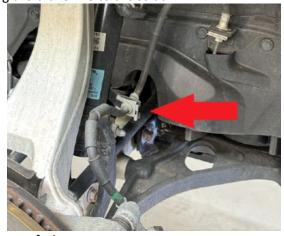
Step 4. Remove bolt holding strut fork to strut.
