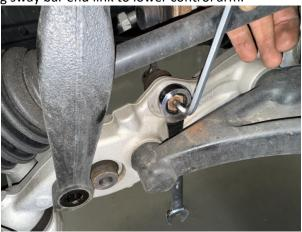
Step 7. Push suspension assembly downward to release strut fork from lower control arm.
