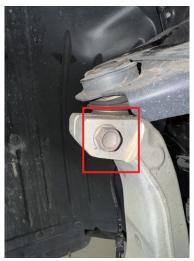
Step 3. Remove C-clip holding the brake line to the strut.
