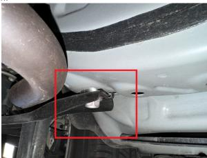
Step 25. Locate 19mm nuts on main subframe studs, loosen, do not remove both rear nuts, allowing subframe to drop about ¼ inch (6.3mm)
