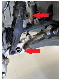
Step 6. Remove bolt holding sway bar end link to lower control arm.
