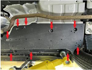
Step 8. Remove plastic aero panels under lower control arms on driver and passenger sides.
