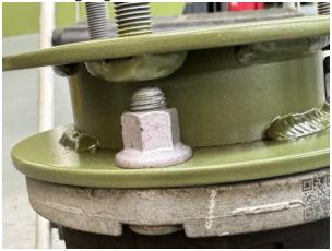
Step 12. Position strut back in shock tower, and loosely install 3 M10 nuts included in the kit to hold it in place but allow some movement until the installation is complete.
