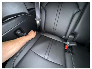
Step 3. Locate rear strut access panels and carefully remove them to allow access to rear strut mounting bolts.
