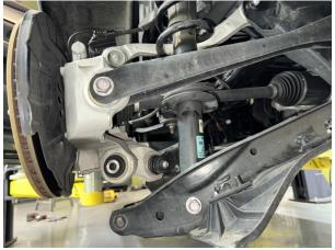
Step 12. Remove lower rear strut bolt.
