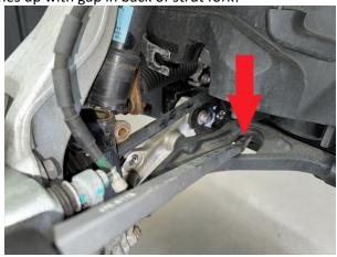
Step 14. Reinstall bolt holding strut fork to strut.
