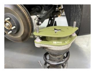
Step 16. Position strut in place and attach strut to lower control arm.
