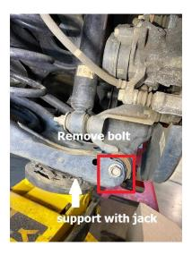
Step 6. Release pressure on spring by lowering control arm with floor jack. It may be necessary to loosen the bolt on the inner end of the rear lower control arm to allow the arm to fully drop.
