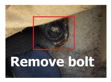
Step 4. Lift up rear seat back to remove, exposing rear strut mounting bolts. These will be removed in step 9.
