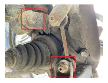
Step 9. Remove 3 nuts holding strut to rear shock tower.
