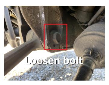
Step 7. Remove driver side rear sway bar end link.
