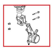
Step 8. Using a length of wire, or large zip ties, secure wheel hub so as to prevent axle shaft from slipping out of inner joint.
