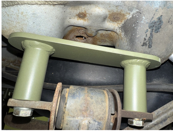
Step 26. Install parking brake cable bracket with M8 bolt (see photo)
