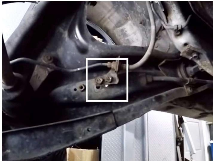
Step 16. Drill a mounting hole in the upper edge of the trailing arm for the rear brake line bracket.
