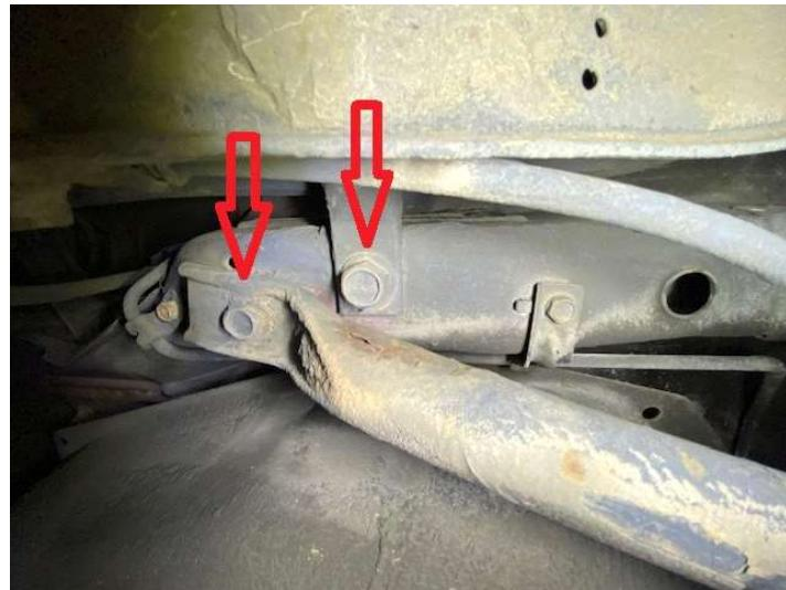
Step 14. Install 1.25x1.5" M12 spacers and M12x90mm bolts one at a time in rear trailing arm to frame.
