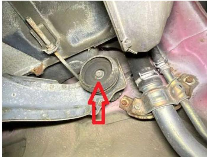
Step 8. Install 2 2.5x1" spacers between rear differential support bracket and chassis. Replace OEM bolts.
