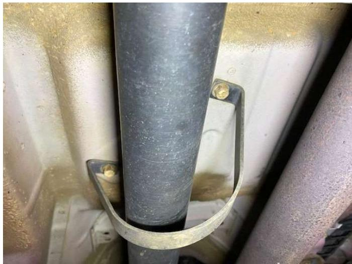
Step 10. Support propeller shaft with floor jack, carefully remove 2 14mm bolts holding center carrier bearing on propeller shaft.
