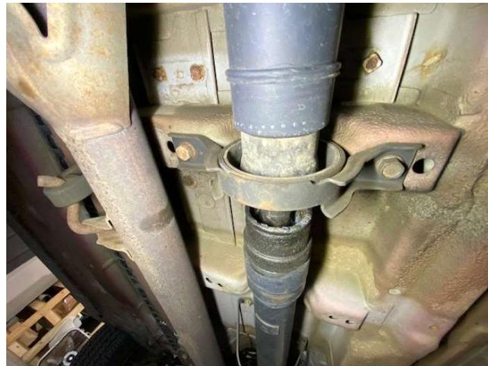
Step 11 Install (2) 1x1" M10 spacers and 2 M10x50mm bolts between carrier bearing and body.
