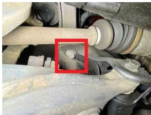
Step 8. Remove cruise control module (if applicable) to gain access to driver side engine mount.
