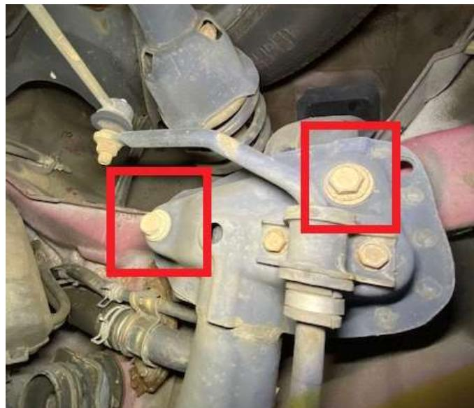
Step 5. Install 4 1.25x1" M12 spacers between cross member and chassis using M12x110 bolts. Install new bolts one by one to maintain alignment of crossmember.
