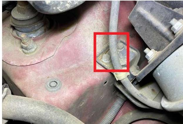
Step 9. Remove 17mm bolts and nuts holding bracket to frame rail and engine mount.
