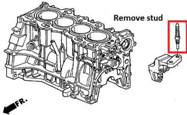
Step 12a. For automatic RT4WD and 2WD transmissions: Remove 1 17mm bolt and 2 17mm nuts on transmission mount, remove bracket.
