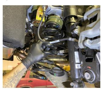
Step 26. Using a floor jack, lift lower control arm into position to line up bolt hole on shock.
