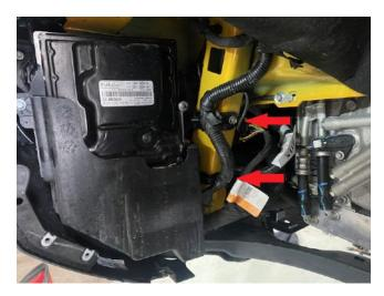
Step 15. Remove intercooler support brackets on both driver and passenger side. (these will be replaced with longer ones) Save hardware.
