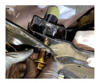
Step 27. Place 4 1x1 M10 spacers between subframe support brackets and body, install 4 M10x50 bolts.
