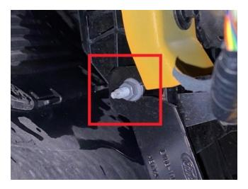
Step 16. There is one bolt on the bottom of each side and 2 nuts in the front of each side. (see photos) Remove lower bumper support bar
