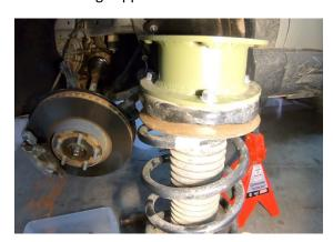
Step 53. Reinstall strut with spacer attached, using original hardware through the shock tower and into the spacer.
