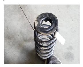
Step 15. Place rubber isolator over rear spring spacer.
