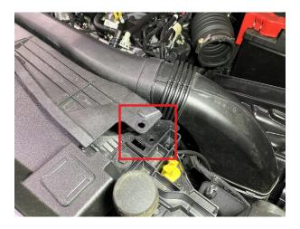
Step 4. Remove air box assembly by pulling upward.
