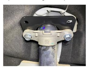
Step 19. Place 2 1.25x1 M12 spacers between shock extension and body, bolt to body using hardware provided in the kit. (see photo)
