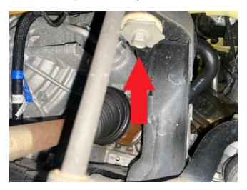
Step 21. Remove 2 M10 bolts located at front of front subframe.
