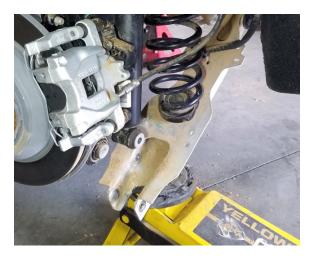
Step 14. Remove spring and upper rubber isolator.
