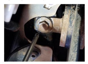
Step 22. Place provided 1.25x1.5 M14 spacers between trailing arm and body.
