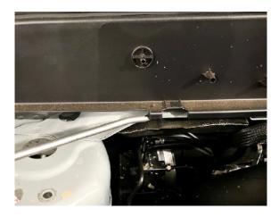
Step 48. Using a 10mm socket, remove plastic panel covering strut bolts.
