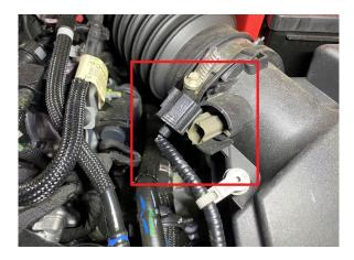
Step 3. Remove 2 clips holding air intake to front support.
