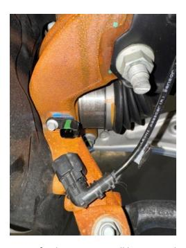
Step 51.Remove ABS wiring from inner fender. ABS wire will be rerouted and plastic clips will not be reused.
