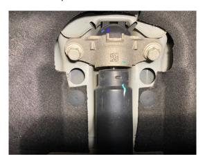
Step 17. Remove 2 bolts holding rear shock to inner fender, remove shock.
