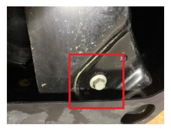
Step 22. Remove Torx screws holding heat shield in place. (see photo below)
