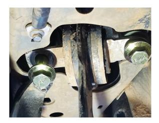
Step 24. Reinstall felt liner.
