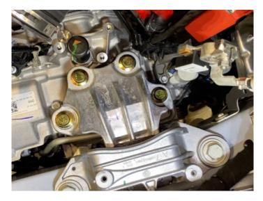
Step 38. Place 4 1.25x1 M12 spacers between engine bracket and engine. Install 4 M12x80 bolts.
