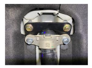
Step 20. Fold back felt liner to access trailing arm mounting bolts.
