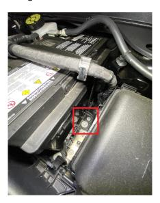
Step 2. Disconnect air intake temperature sensor.
