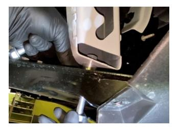
Step 30. Install "S" brackets in place of OEM intercooler support brackets, secure with factory hardware.
