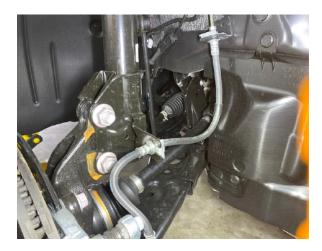
Step 5. Remove 17mm nut holding sway bar link to strut.
