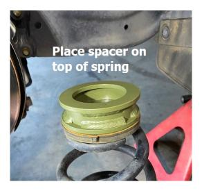
Step 12. Use floor jack to compress the springs and raise the rear axle back into place.
