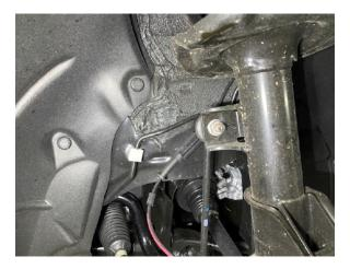
Step 6. Remove 2 21mm nuts from strut mounting bolts, slide bolts out. It may be necessary to tap these bolts out with a hammer.
