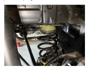
Step 13. Remove bolts holding shock into rear shock tower.
