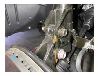
Step 11. Leave sway bar link loose until both sides are complete.
