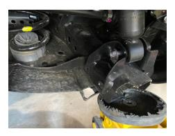
Step 7. Unclip rear brake line and unbolt ABS wire.
