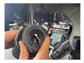
Step 11. Place lift spacer between frame rail and isolator, reinstall spring.
