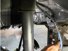
Step 8. Release pressure on springs by lowering rear axle with floor jack.
