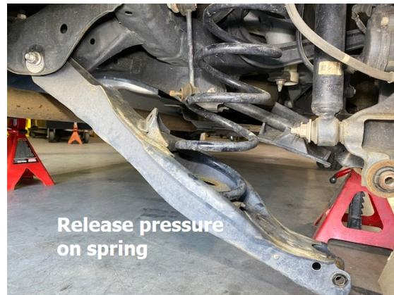
Step 7. Remove spring and rubber isolator.
