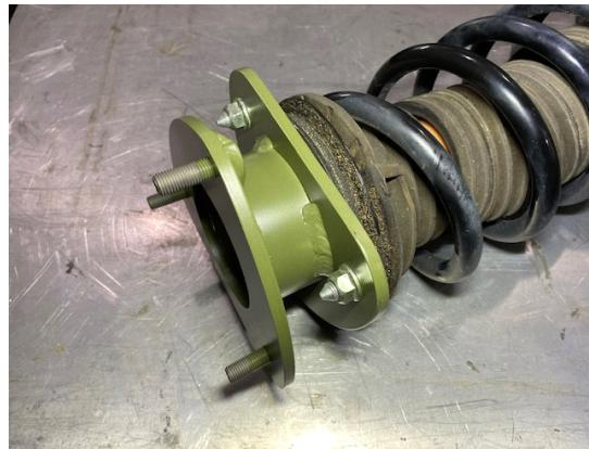
Step 8. Slide lift spacer through bolt holes in strut tower. Secure with OEM hardware.
