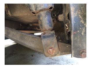
Step 5. Remove 2 14mm nuts at the top of the strut connecting the strut to the strut tower, remove strut. Save hardware for reinstallation.
