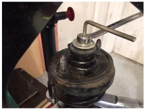
Step 9. Using a bench grinder, remove approximately 1/8" from the end of the top hat studs. Test the fitment and be sure the studs do not protrude past the top of the spacers.
