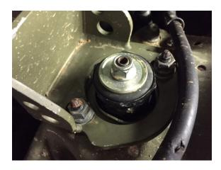
Step 8. Mark spring orientation on top hat. Using spring compressor, remove top hat from strut. use 4mm hex key to hold strut shaft while loosening nut. Inspect strut and bump stop, replace if necessary.
