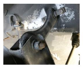
Step 4. Remove 14mm bolt connecting strut to lower control arm. Save hardware for reinstallation.
