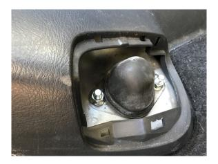
Step 6. Install lift spacers onto struts using original hardware. (See diagram)
