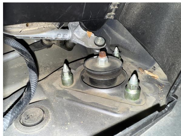
Step 2. Remove nuts holding driver side strut to shock tower, leave one nut on so struts do not fall when lifting vehicle to access bottom bolts. Save hardware.
