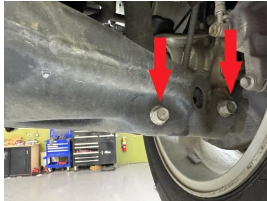
Step 6. Using a floor jack, carefully lower rear control arm to release pressure on spring.
