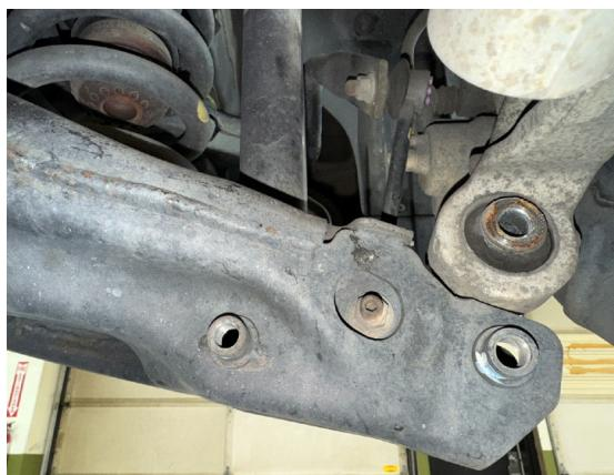
Step 6. Pivot lower arm down enough to remove spring. (see diagram below)
