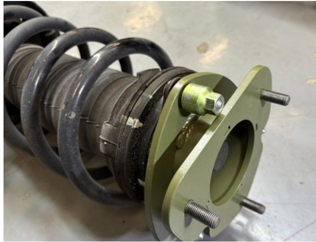
Step 12. Reinstall strut in reverse order, using supplied hardware to bolt strut to body.
