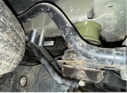
Step 7. Place 1.25x2 M12 spacers between subframe support brackets and body, install 8 M12x70 bolts.
