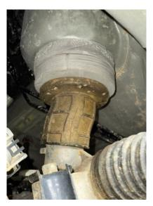
Step 15. Under driver side dash, remove plastic dust cover on steering column. Trim away plastic as necessary to eliminate contact with steering shaft.
