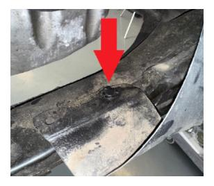
Step 12. Re-install aluminum heat shield, drill new holes and bend as necessary to fit with lowered subframe. Re-attach using OEM hardware.
