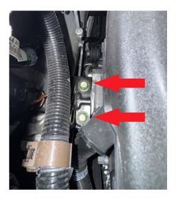
Step 2. Remove bolt on rear outer corner of air box (see photo)
