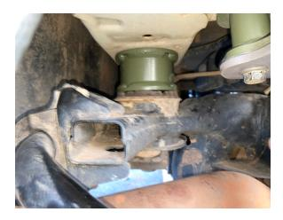
Step 6. Remove rear subframe bolts one by one, installing remaining 3.5x2" spacers and installing M14x180 bolts. (see photos)
