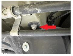
Step 14. Place 3 0.75x1 M8 spacers between gas tank bar and body, install 3 M8x40 bolts.
