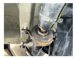
Step 12. Remove bolts holding plastic under tray to gas tank bar (save hardware).
