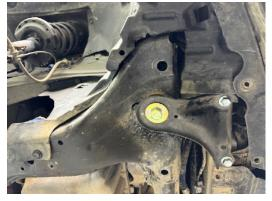
Step 11. Trim fender liner as necessary to fit with lowered subframe, relocate flap to top side of subframe and secure using original hardware. (see photo)
