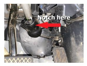
Step 16. Re-install dust cover on steering column below interior dashboard. Double check full rotation of steering wheel to check for any noises or rubbing. Trim as necessary.
