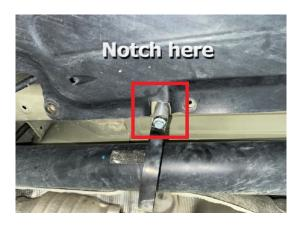
Step 10. Remove 2 M10 bolts holding driveshaft carrier bearing.
