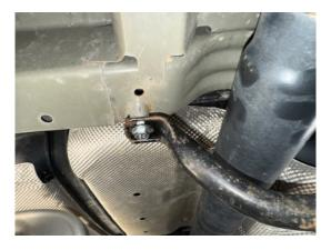
Step 15. Remove tailpipe hangers from tailpipes.
