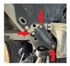
Step 9. Remove the 2 remaining OEM subframe bolts one at a time, lower subframe carefully about 2 inches with floor jack or screw jacks and slip 2.75x2 M14 spacers between subframe and body, installing M14x180 bolts as you go. (This keeps the subframe square and aligned during installation.)
