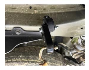
Step 17. Install extended exhaust hanger in place of center exhaust hanger (see photo)]
