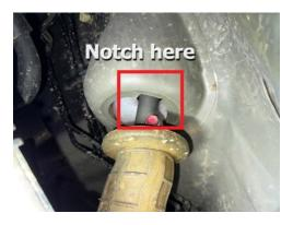
ALTERNATE METHOD: Using a screwdriver or round bar, bend sheet metal back about 1/4 inch around the coupler. Turn steering wheel to verify the coupler has proper clearance.
