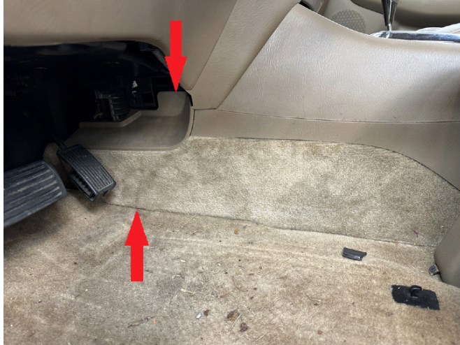
Step 12. Under driver dash, remove plastic cover, disconnect light
