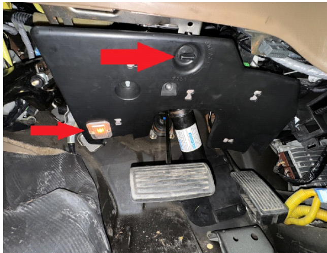
Step 13. Remove plastic cover over steering column.
