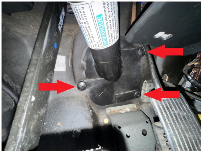
Step 14. Using a body saw, trim sheet metal for clearance around steering coupler. This can also be done
