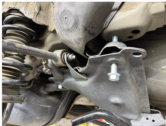
Step 9. Remove M12x100 bolt from previous steps and place 1.25x1 M12 spacer between subframe and chassis on driver side front corner. Permanently install bolt. Repeat for remaining 3 subframe bolts. Torque to 76 ft-lb.
