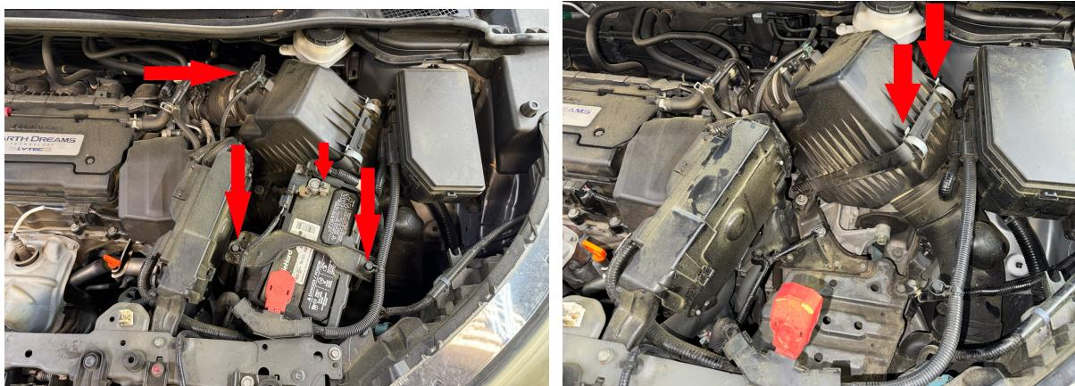
Step 3. Remove the ECU support bracket.
