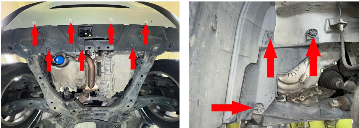
Step 10. Starting with the driver side front, Remove the main subframe bolt and temporarily replace with an M14x150 bolt. Repeat for passenger side front bolt.
