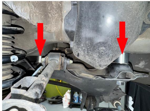
Step 10. Remove M10x140 bolt holding rear differential bracket to chassis and place 2.75x1 M10 spacer between differential bracket and chassis. Permanently install bolt. Torque to 49 ft-lb. Repeat for remaining bolt.
