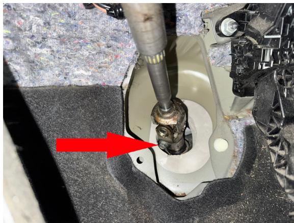
Step 24. Re-install dust cover on steering column.
