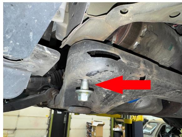
Step 11. Remove rear most bolts on front subframe one at a time, replacing with longer bolts included in the kit.
