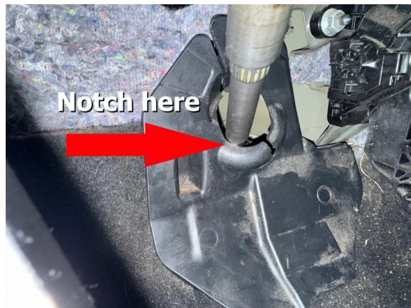
Step 23. Rotate steering wheel to check for noises. If noise is present, loosen M8 bolt 2 turns on steering "U-joint" couplers, turn the wheel lock to lock and then re-tighten. **Do not remove these bolts!**
