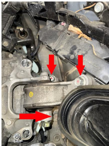
Step 17. Place 2 "stepped" 1.25x1 M12 spacer over studs. (see photo)
