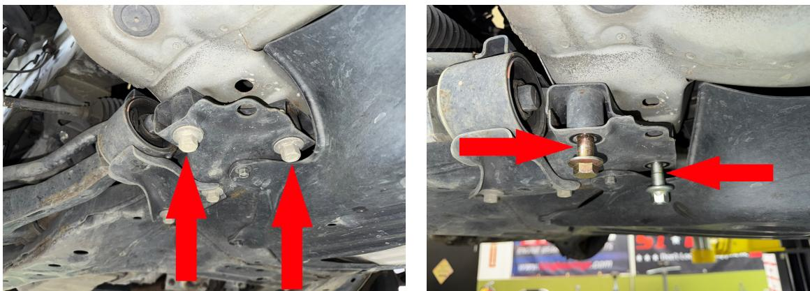
Step 12. Locate and remove subframe bolt in wheel well. Repeat for opposite side.
