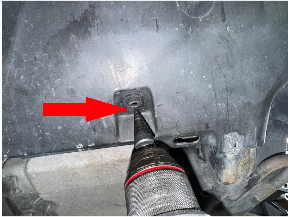
Step 22. Trim plastic splash shield as shown to fit with lowered subframe, reinstall using original hardware.
