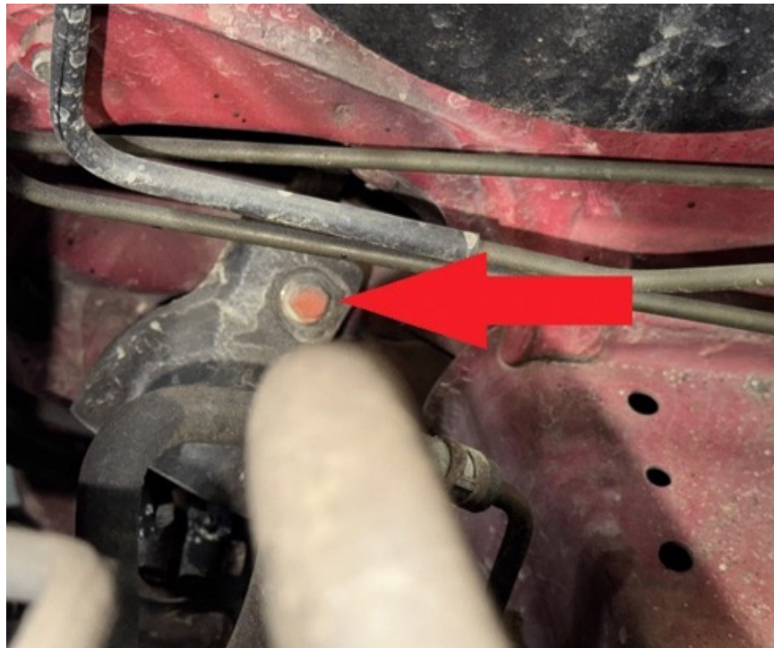
Step 26. Remove 4 12mm bolts holding driveshaft safety loops to body. Install 4 0.75x1" spacers and M8x40 bolts as shown.
