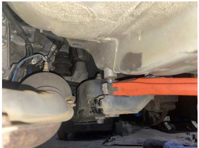
Step 13. Carefully lower front subframe as needed to pull stud out of its location. ALTERNATIVE METHOD: Cut the stud in half to make it easier to remove.
