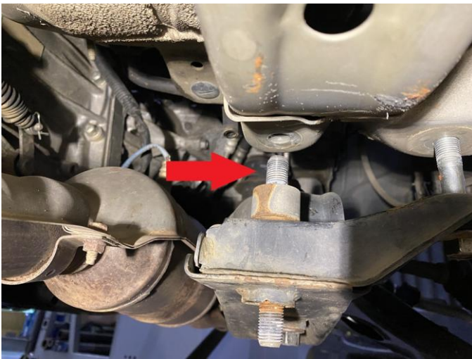
Step 13. Carefully lower front subframe as needed to pull stud out of its location. ALTERNATIVE METHOD: Cut the stud in half to make it easier to remove.
