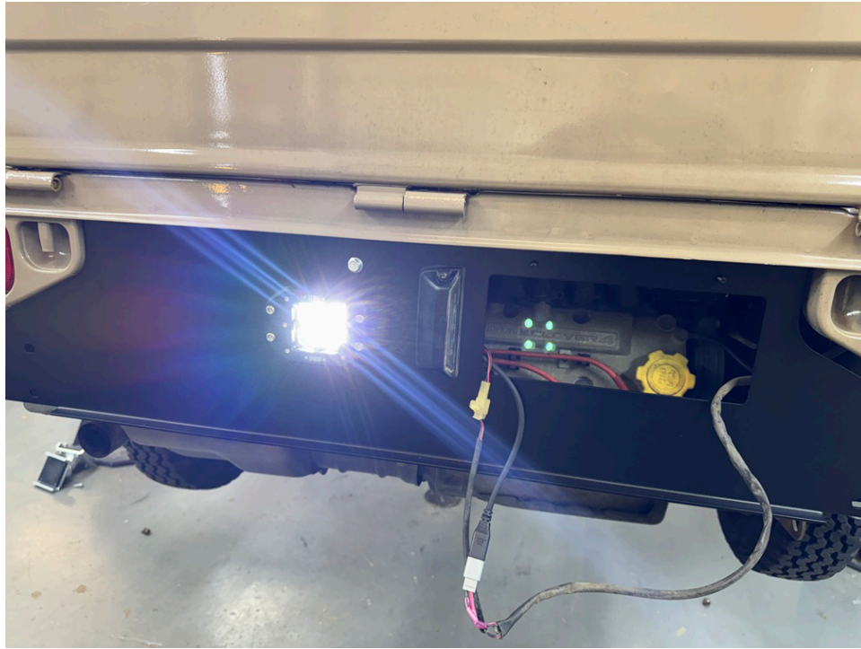
Step 17. Zip tie the wiring into a bundle and then zip tie to the existing wiring harness as shown.
