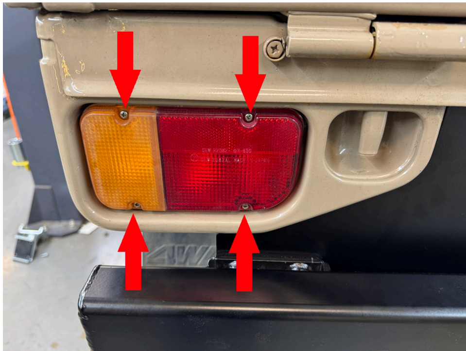
Step 20. Using a 14mm ratcheting wrench, install remaining M10 nuts.
