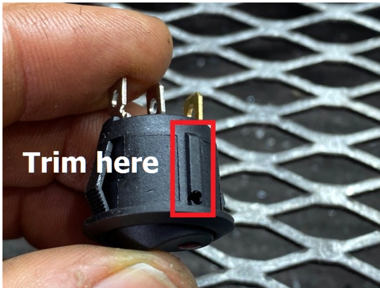
Step 21. Using a utility knife, trim mounting switch as shown:
