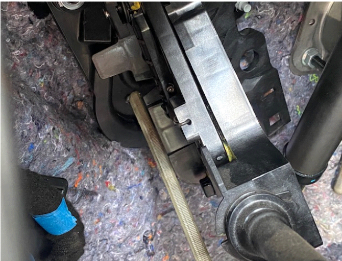
Step 12. Using a wire fish tool, pull switch wiring through firewall.
