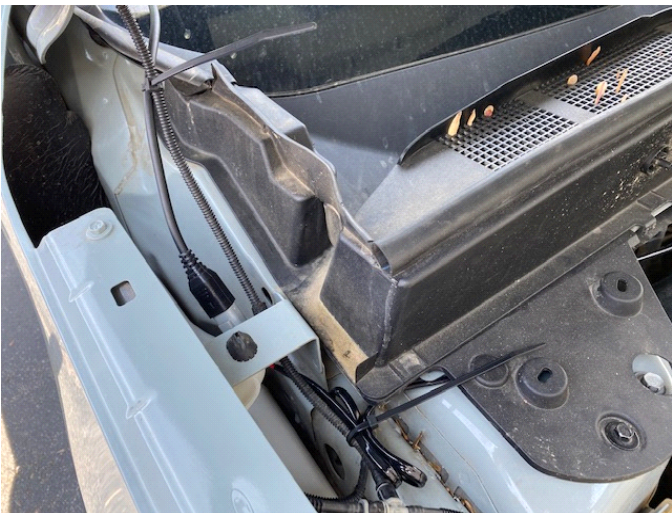
Step 28. Route wiring to lights as shown, secure with cable ties:
