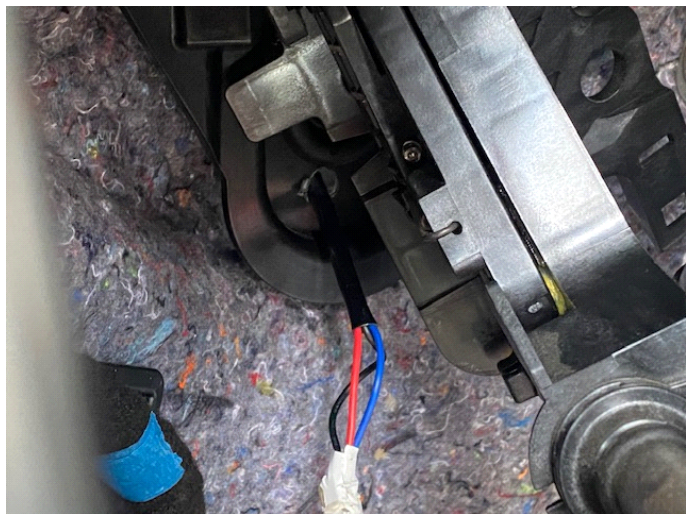
Step 14. Choose a suitable location to mount power switch. It can be mounted wherever you like. (We mounted ours to the light control panel)
